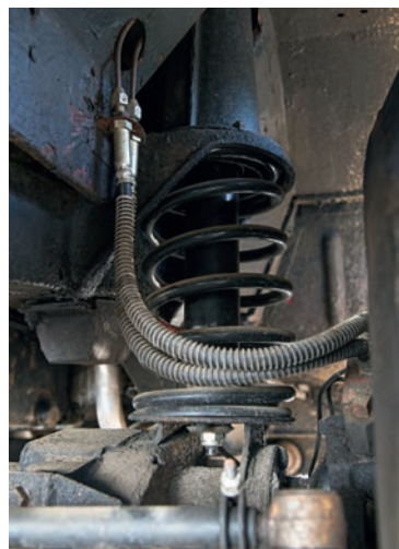
Long-travel coil-sprung suspension was a revelation off road compared with a leaf-sprung set-up; it was petrol only until 1986
