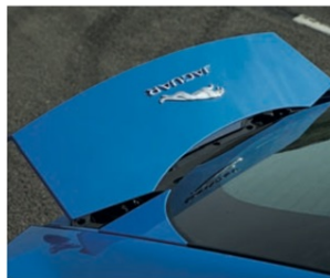
Deployable spoiler ascends at high speeds
