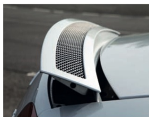
Audi's meshed grille reduces drag further
