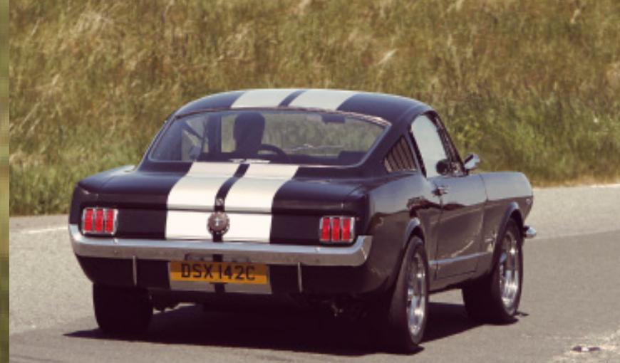
Body movements are well controlled, but the live rear axle can cause mid-bend skips
